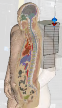
Numerical simulation of the health risks of a man-portable transmitter
