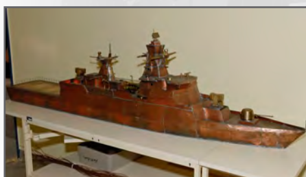
Scale model for the verification of numerical simulation codes
