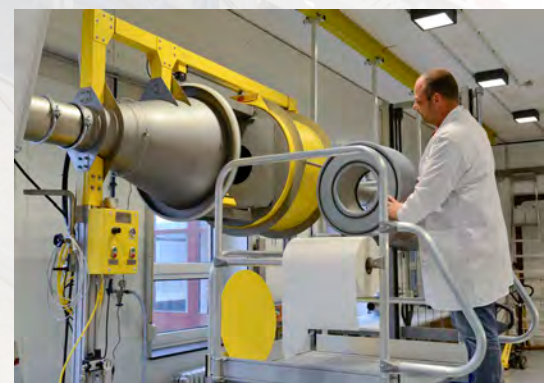
Testing of permeability of filter with aerosol
