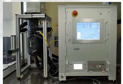
Magnetic suspension balance for the generation of highly diluted CWA containing test gases.
