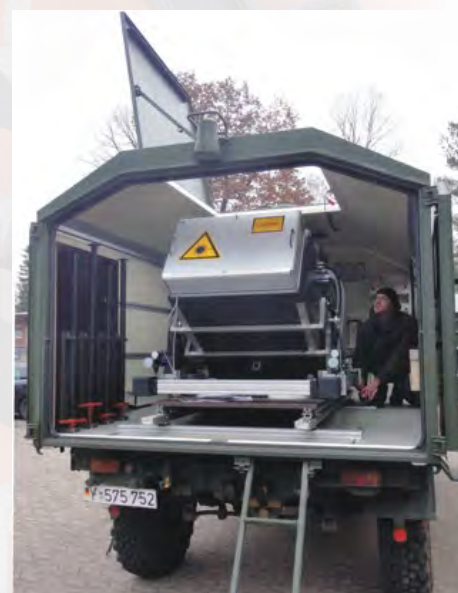
Pivoting device laser unit BALL and its integration into a BW vehicle 2t
