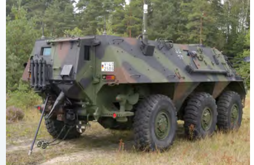
Rear view of the FUCHS NC-reconnaissance vehicle with extended probe and double wheels
