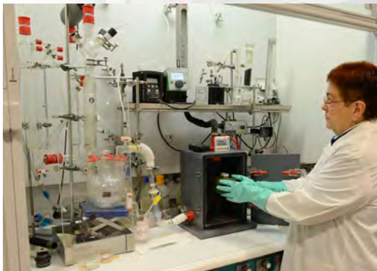
Hydrocyanic acid test stand for filters
