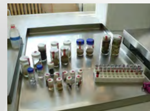
Suspect sample of a fact-finding mission (soil, textiles, rubber, organic solvents) prior to sample preparation and analysis
