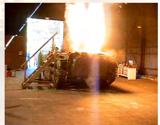
Standardized deflagration used to test various automatic fire suppression systems
