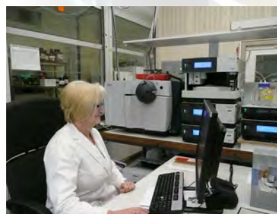
Trace analysis of warfare agents in aqueous solutions using UHPLC-MS (ultra high performance liquid chromatography mass spectrometry)
