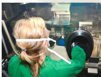
Propagation of monkeypox virus, work in a glove box of safety level 3
