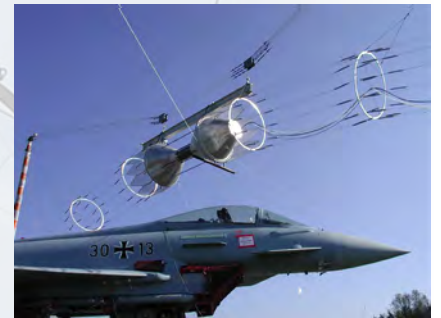
NEMP qualification test Eurofighter (hybrid dipole antenna)
