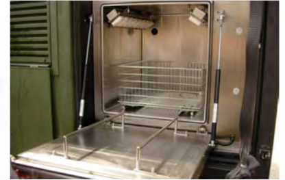
Decontamination of sensitive equipment – vacuum chamber
