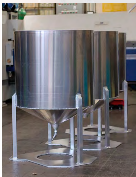
Container for the determination of the air to water ratio of medium expansion foam
