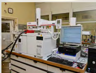
Analysis of VOC using thermodesorption and GC-MS (gaschromatography / Mass spectrometry)
