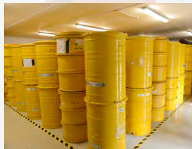
Stored 200 l drums containing radioactive waste
