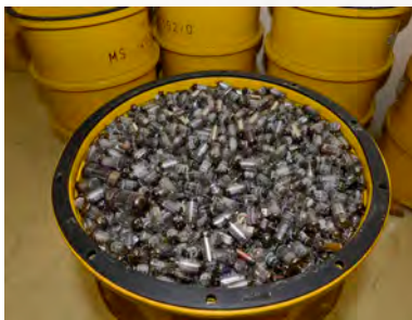
200 l-drum with electronic components which used radionuclides for pre-ionization
