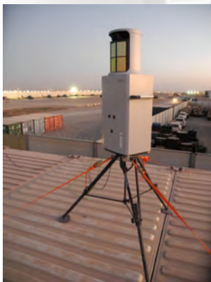
Stand-off detection system SIGIS II after testing and commissioning by WIS 230 during a field operation.
