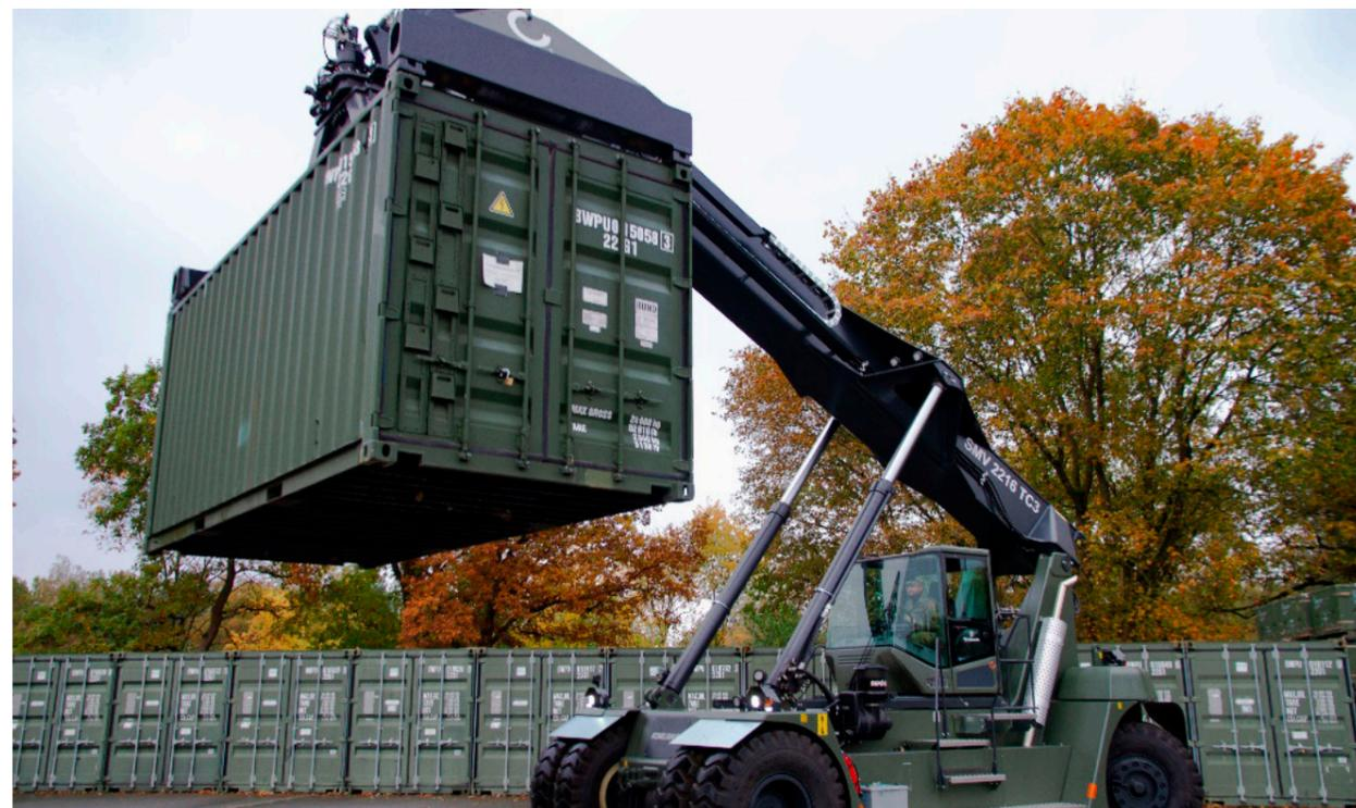
Reach stacker container handler in operation: For the transshipment of material, field handling equipment, or (fork) lift trucks/container handlers, of different working loads are used.
