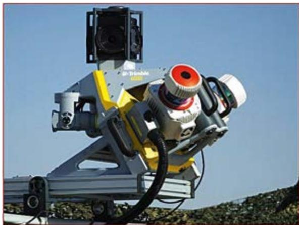
△ Multisensorsystem Trimble MX9. (Quelle: ZGeoBw)
